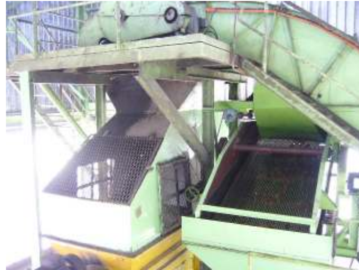
Two-Step Trash Removal
